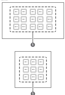
Macro Buttons: Each button contains 2 colour LEDs (red and blue) with adjustable individual brightness levels from 0~100. Each button can activate a customised macro. (For further detail on these settings please refer to section 6.5 "WebGUI Control".)
