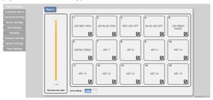
There are 6 macros defined by default for testing the Wall Plate Control System's functionality. Click on macros 1~6 to demonstrate various LED light commands.
