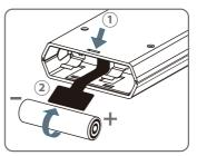
press down into the slot (1) behind the base panel and the bottom cover will pop out.
